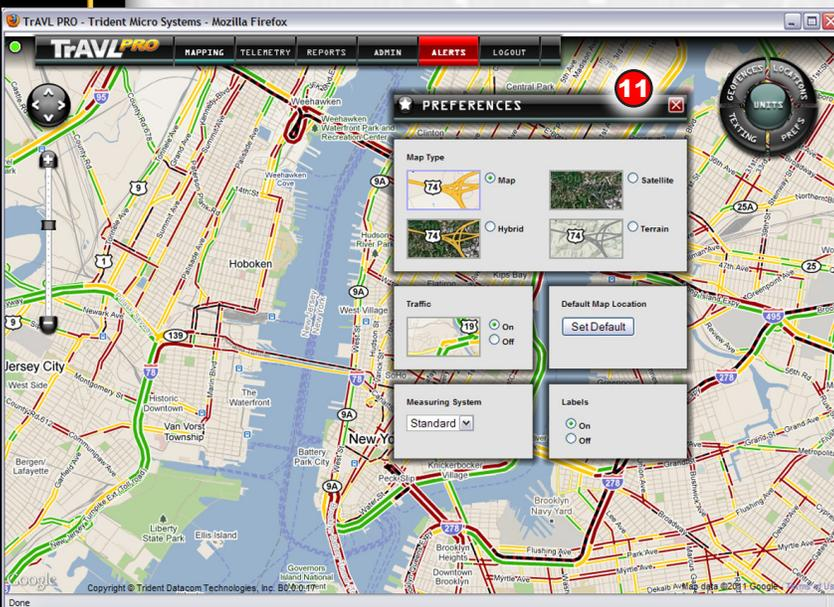
The Preferences (11) window allows for a variety of display settings to be controlled including: Map Type, Traffic, Default Map Location, Measuring System, and Labels On or Off.
